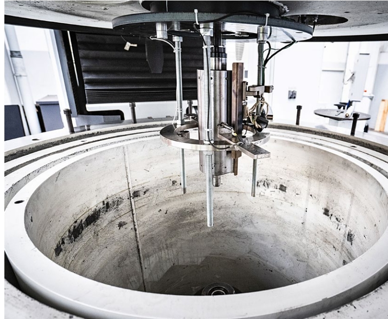
Deep craters on the steel inner walls testify to the extreme forces exerted during testing. Some components are rotated at speeds of up to 200,000 times per minute – until they can no longer withstand the forces and shatter.
