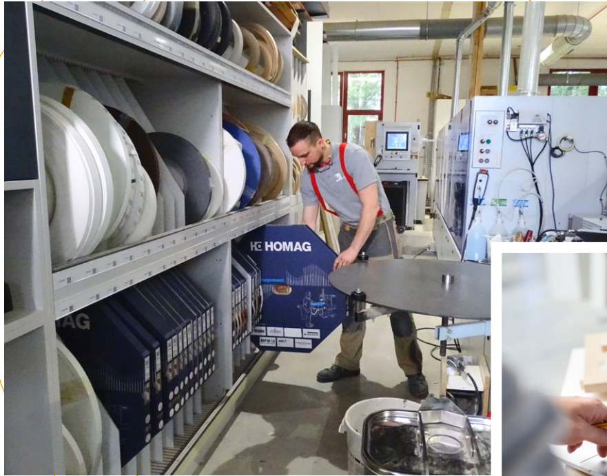
Searching is now a thing of the past: LEDs on the rack indicate in which shelf space the relevant edge banding can be found.
