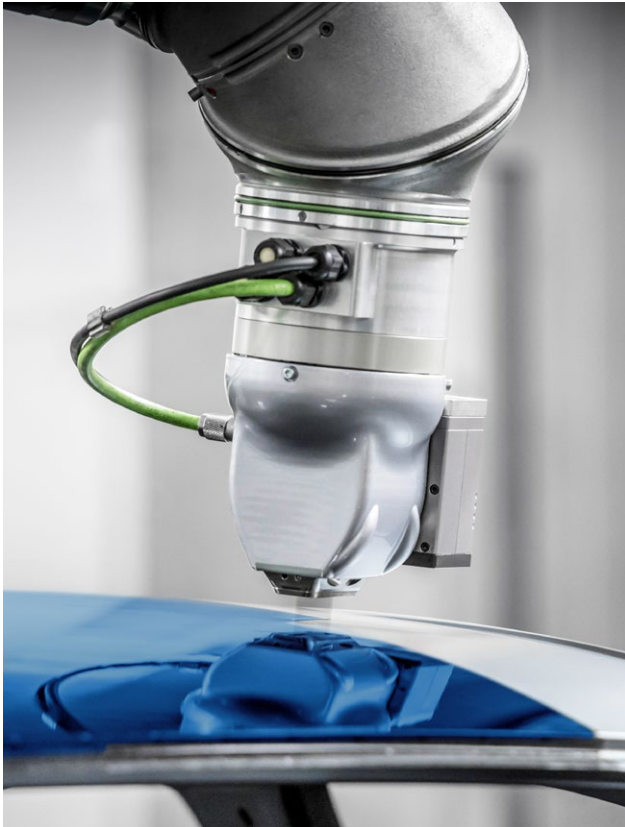
Tiny jets of paint are directed onto the surface. The traditional process, by contrast, atomizes the paint into a mist that cannot be applied sharply.
